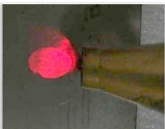
Beam Out of Alignment
