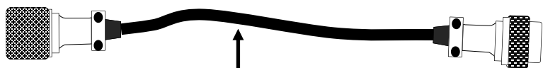
CONTROL ADAPTER FROM DONGLE CONNECTOR TO WELDER (TYPE VARIES BY BRAND, NOT NEEDED FOR SOME APPLICATIONS)
