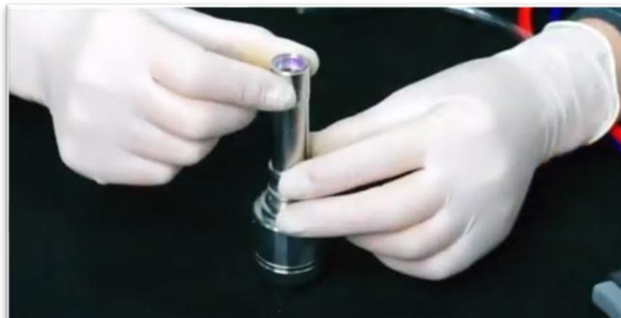
Collimating Lens Assembly Removed from Gun
