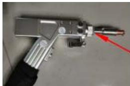
Remove Focus Tube
