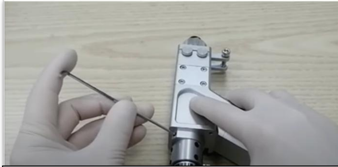
Gun Head Disassembly/Focus Mirror Removal Using Main Set Screw.
