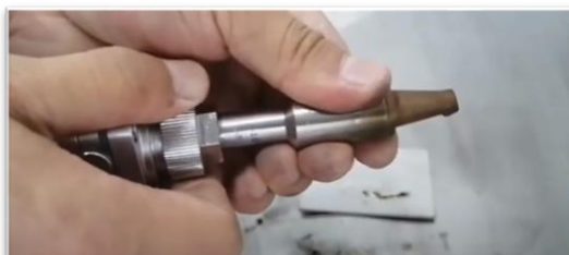
Focus Tube Adjustment
