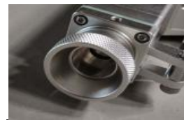
Install Cleaning Nozzle
