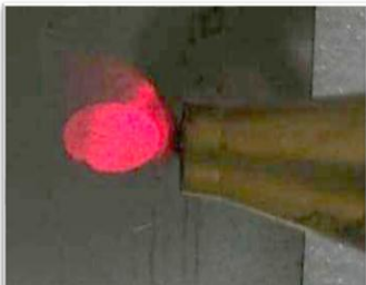
Beam Out of Alignment
